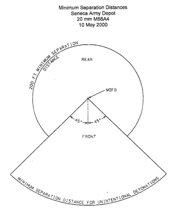
MINIMUM SEPARATION DISTANCE FOR UNINTENTIONAL DETONATIONS USING MINIATURE OPEN FRONT BARRICADE DURING INTRUSIVE ACTIVITIES
