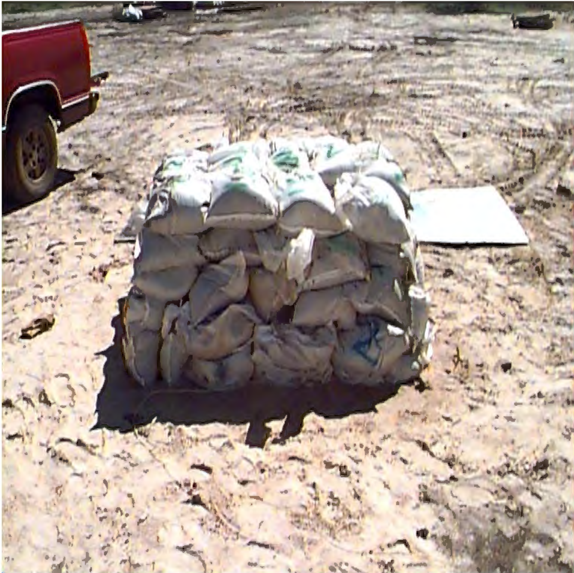
Figure 5 – Sandbag Enclosure for an 81 mm M374A2 mortar.
