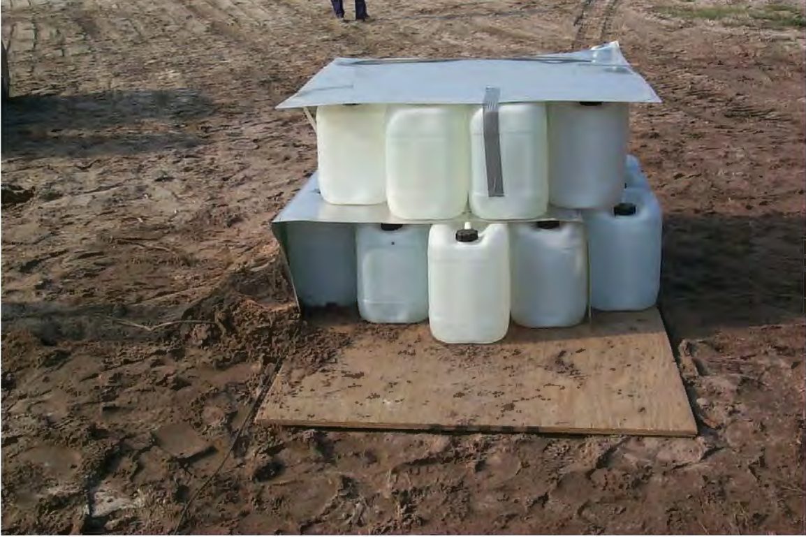
Figure A-22 – Phase 2, 81 mm Under 5 Gallon Carboys Test Set-up
