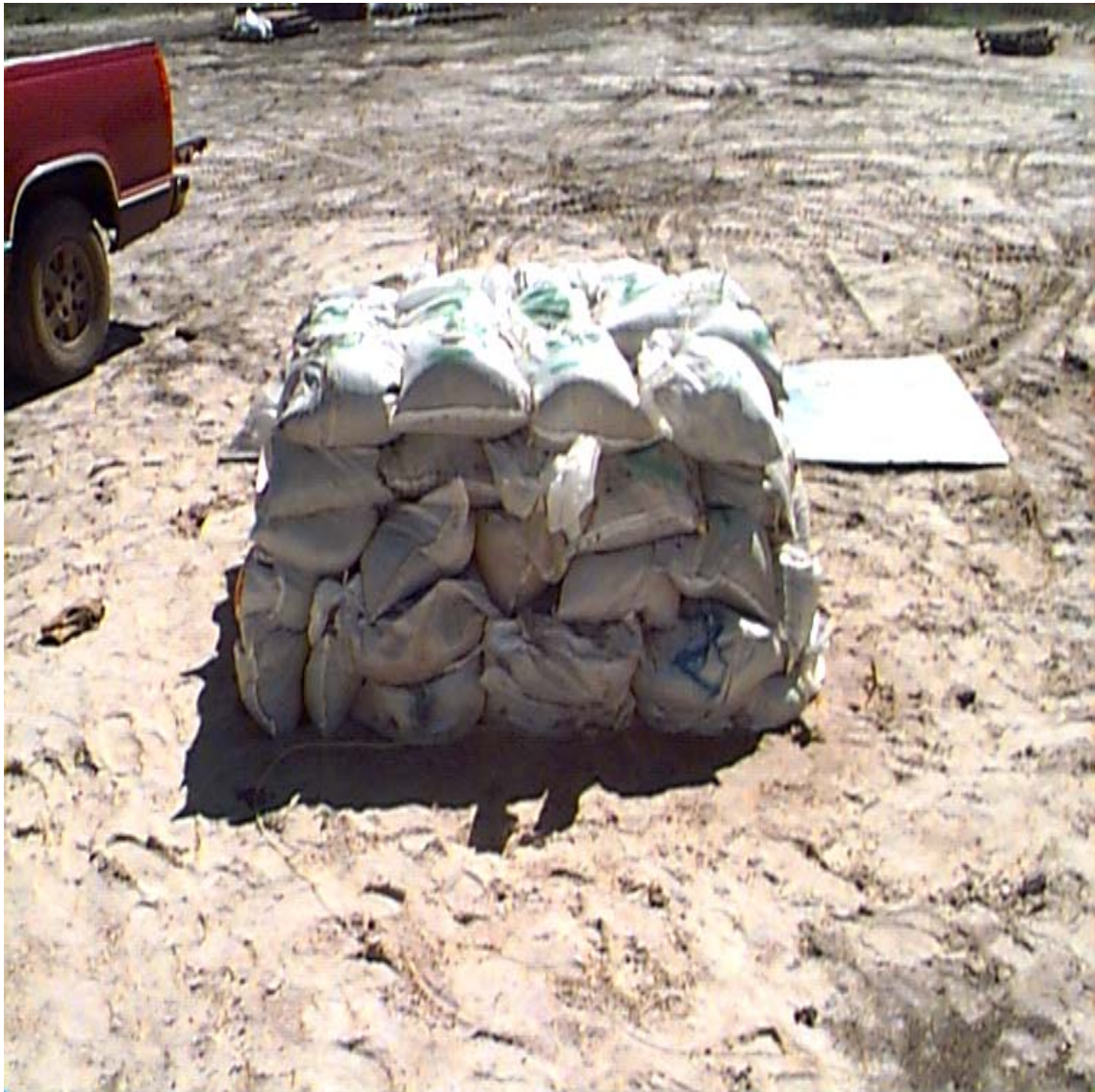
Figure 5 – Sandbag Enclosure for an 81 mm M374A2 mortar.
