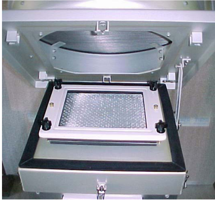
TE-6001 Shown raised over shelter to expose filter cartridge.
