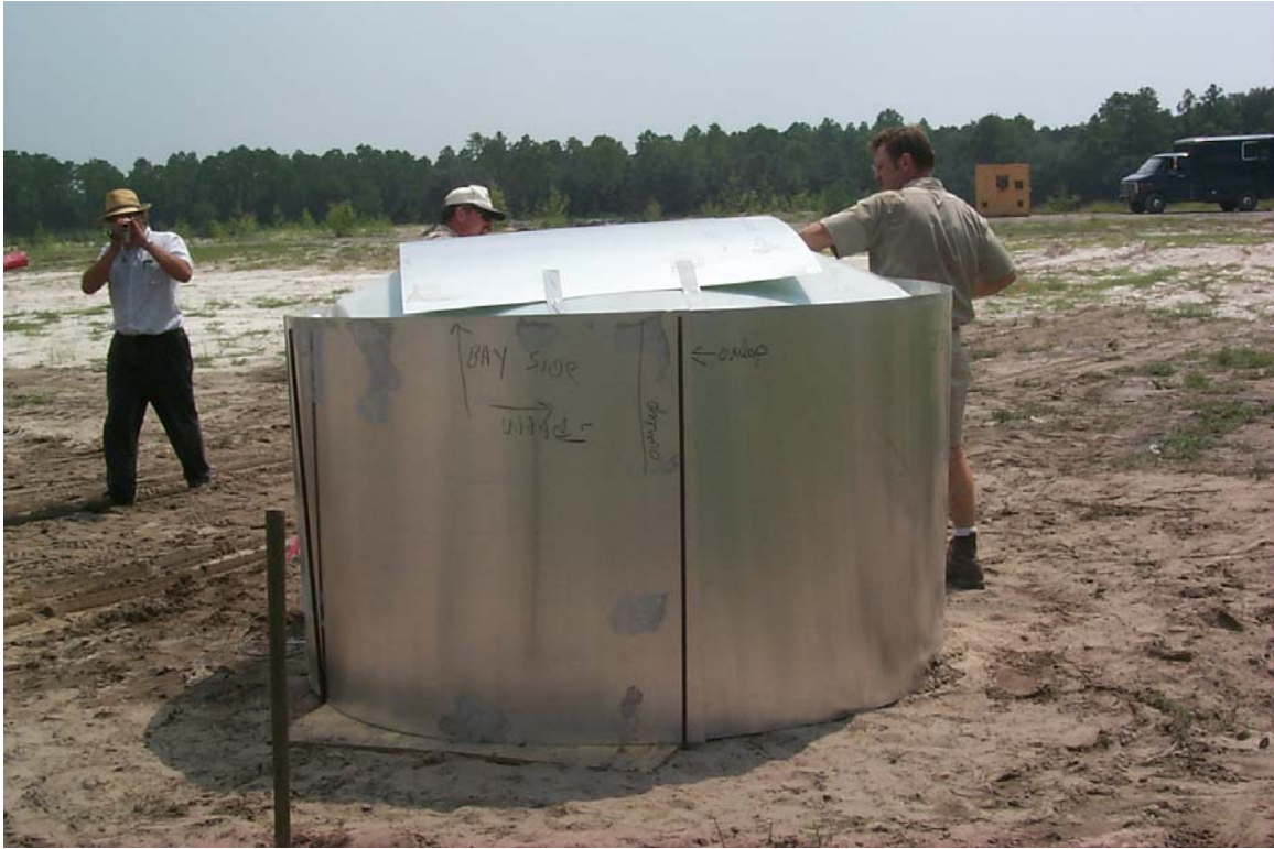
Figure A-14 – Phase 2, 105 mm Under 1100 Gallon Tank Test Set-up
