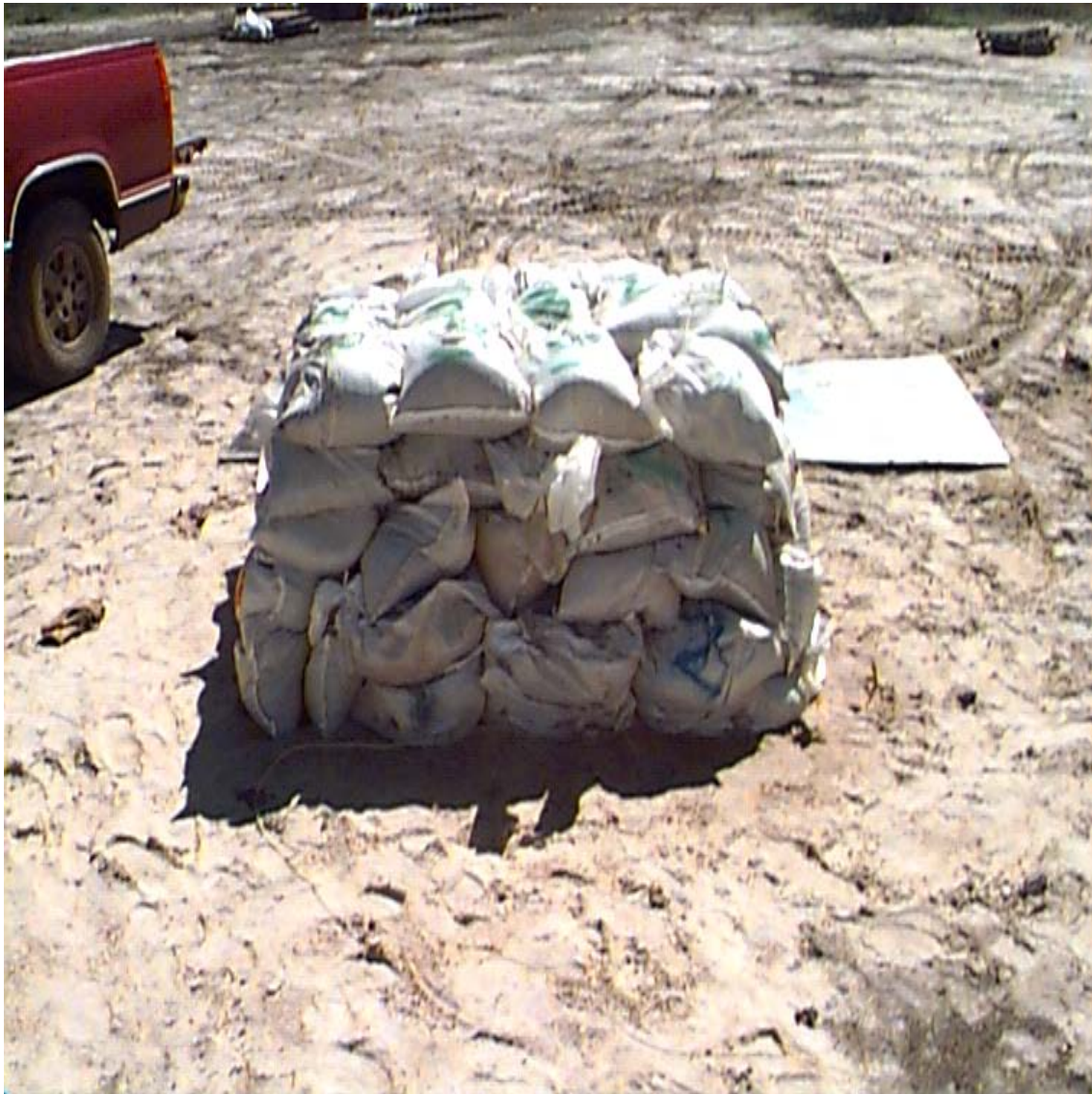
Figure 5 – Sandbag Enclosure for an 81 mm M374A2 mortar.
