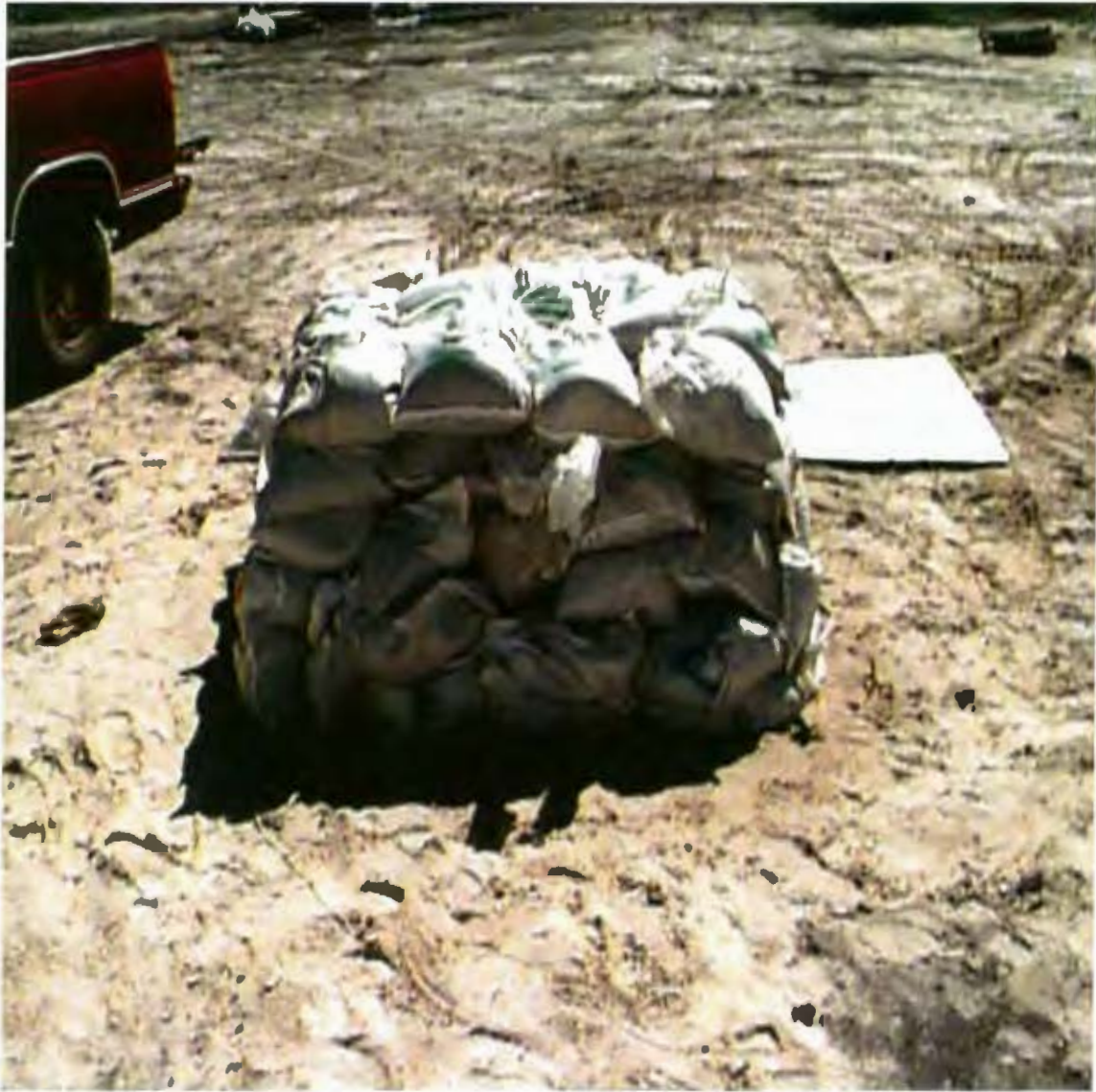
Figure 5 – Sandbag Enclosure for an 81 mm M374A2 mortar.
