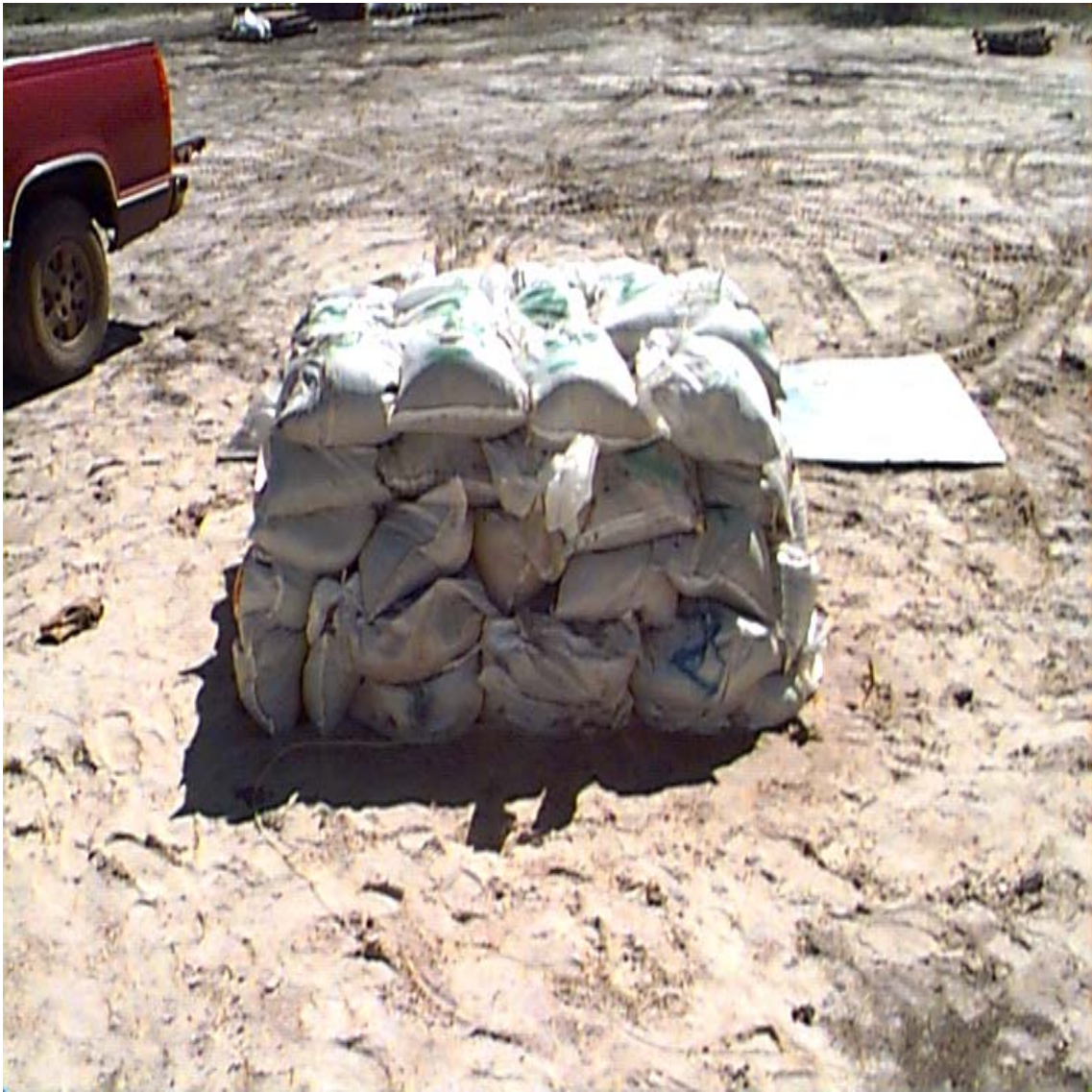
Figure 5 – Sandbag Enclosure for an 81 mm M374A2 mortar.
