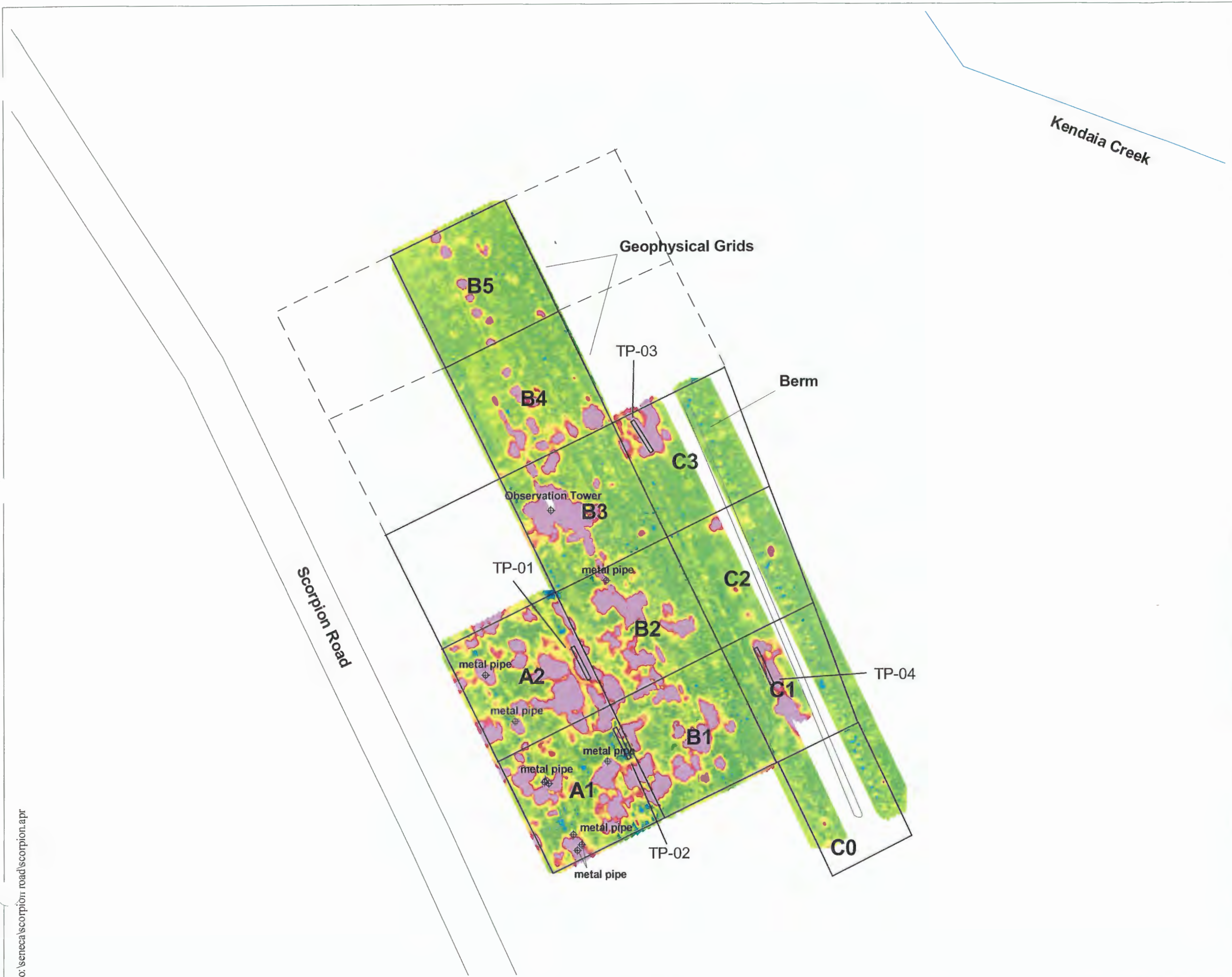
FIGURE 3-2 TEST PIT LOCATIONS VERSUS RESULTS OF GEOPHYSICAL SURVEYS AT THE SMALL ARMS RANGE
