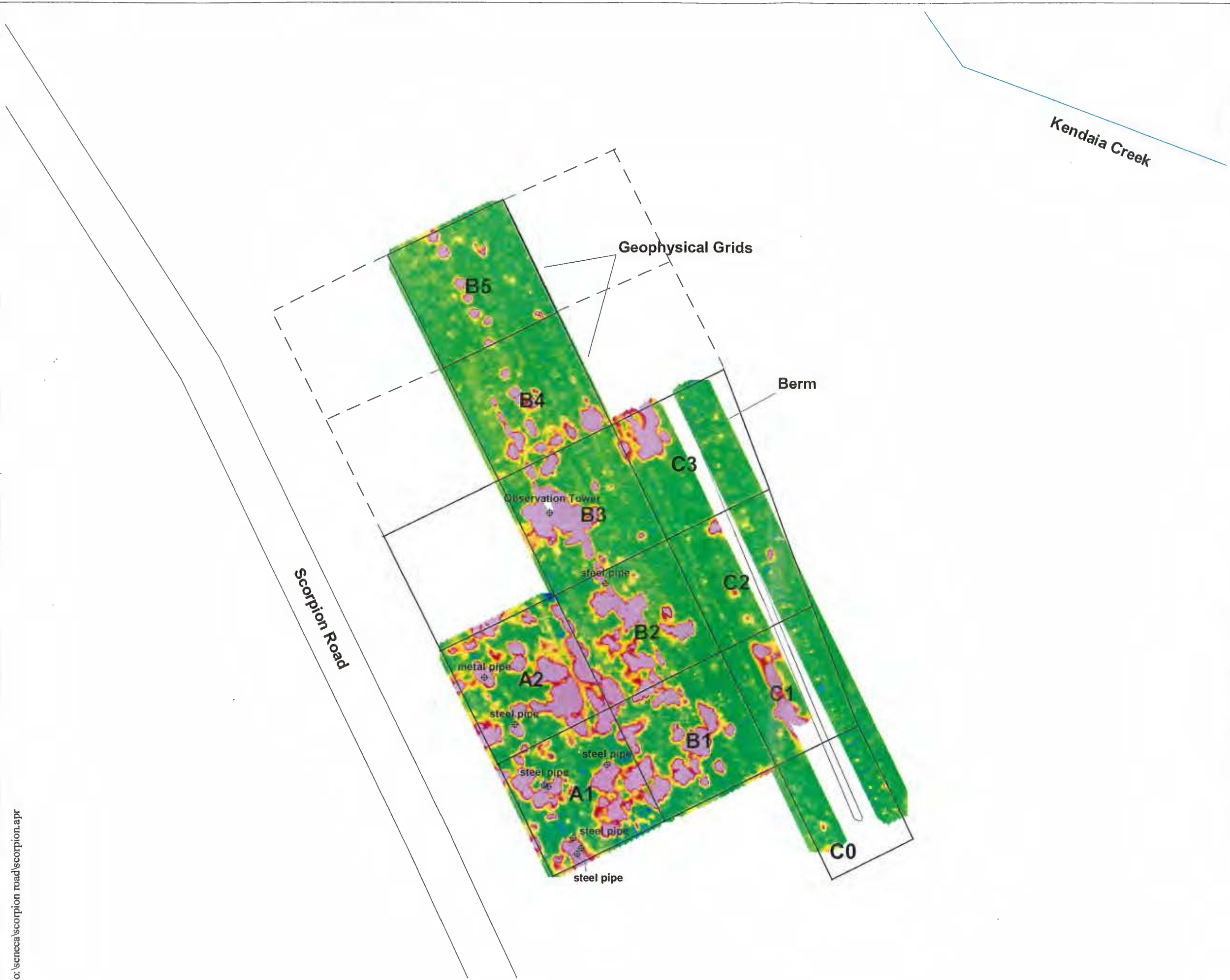
FIGURE 3-1 RESULTS OF GEOPHYSICAL SURVEYS AT THE SMALL ARMS RANGE
