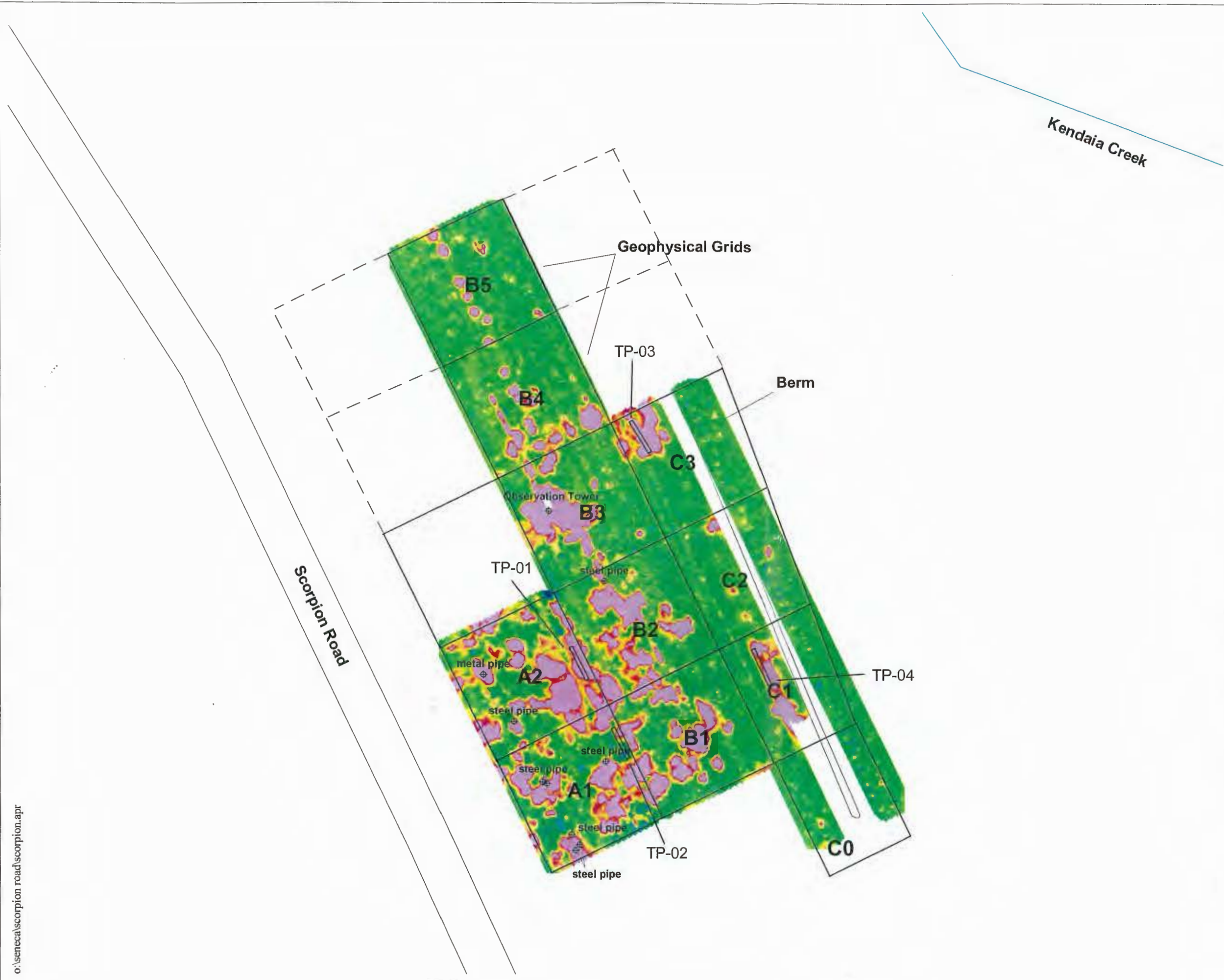
FIGURE 3-2 TEST PIT LOCATIONS VERSUS RESULTS OF GEOPHYSICAL SURVEYS SMALL ARMS RANGE
