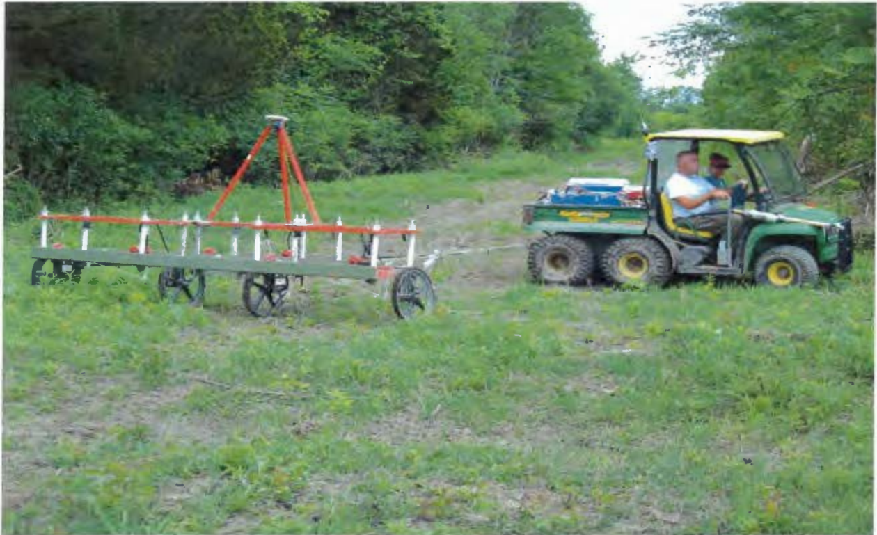
Photo No. 1: EM61-MK2 Towed-Array System (July 2003)
