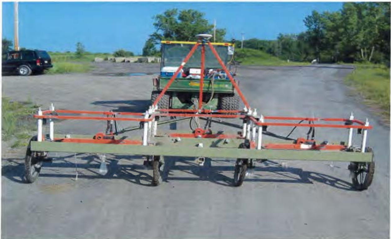
Photo No. 2: EM61-MK2 Towed-Array System (July 2003)
