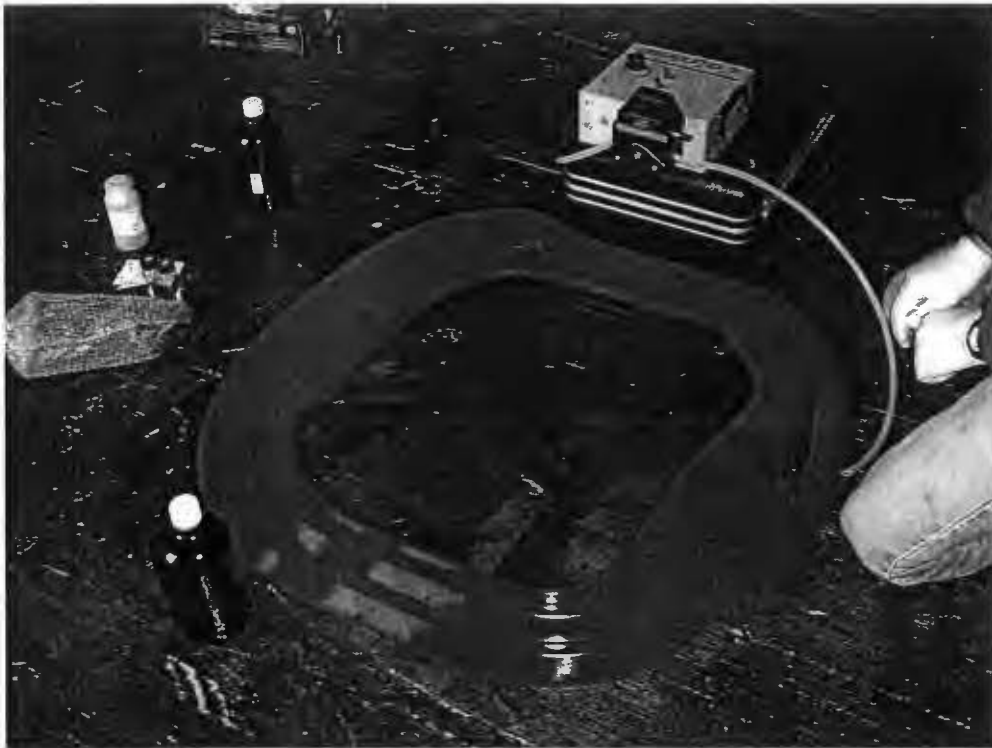
Rinsate dike and collection pump.
