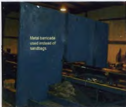
17. Metal barricade used instead of sandbags
