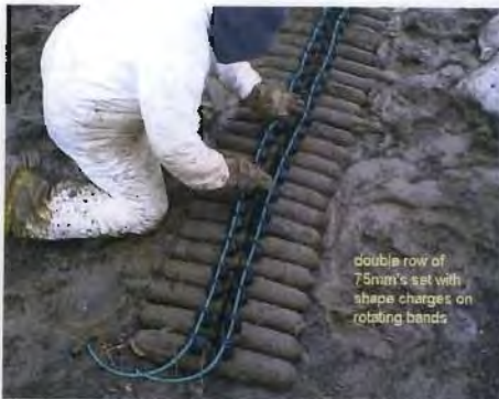
11. Double Row of 75mm Projectiles set With shape charges on rotating bands
