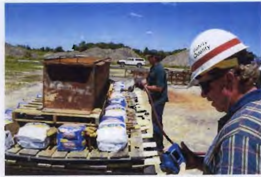
33. OE Material being soaked with diesel
