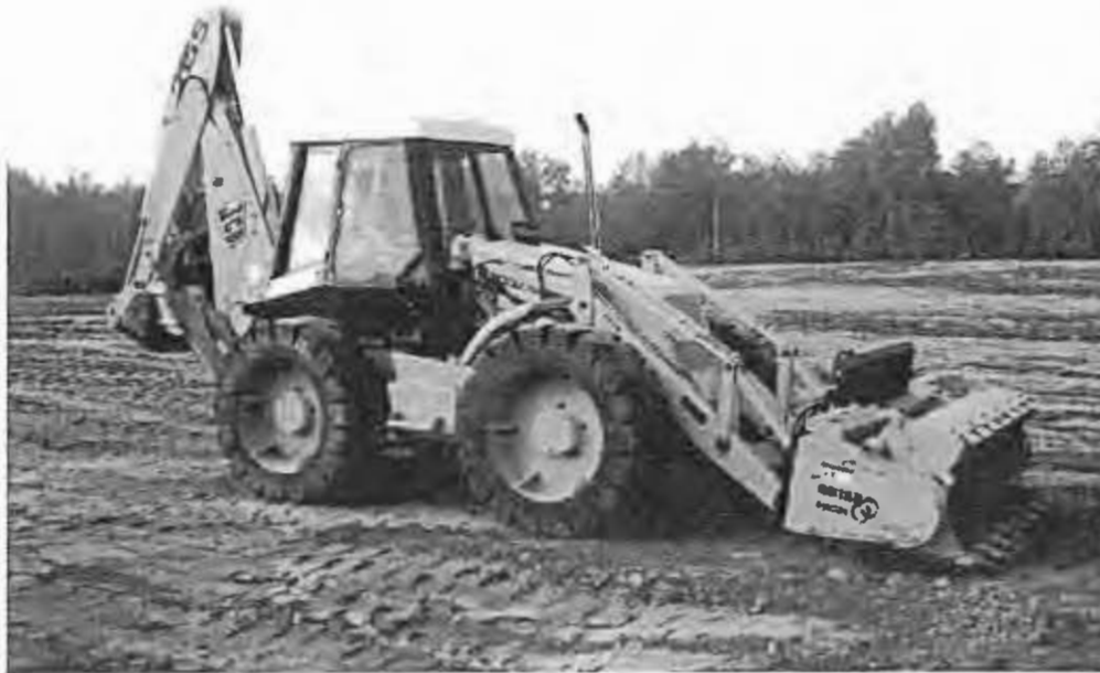
Figure 1. Improved Backhoe With HPL 800 S ROTAR ®
