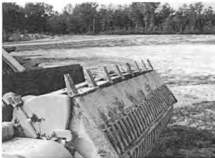
Figure 16. Blast Distortion (Bowing) to ROTAR ®
