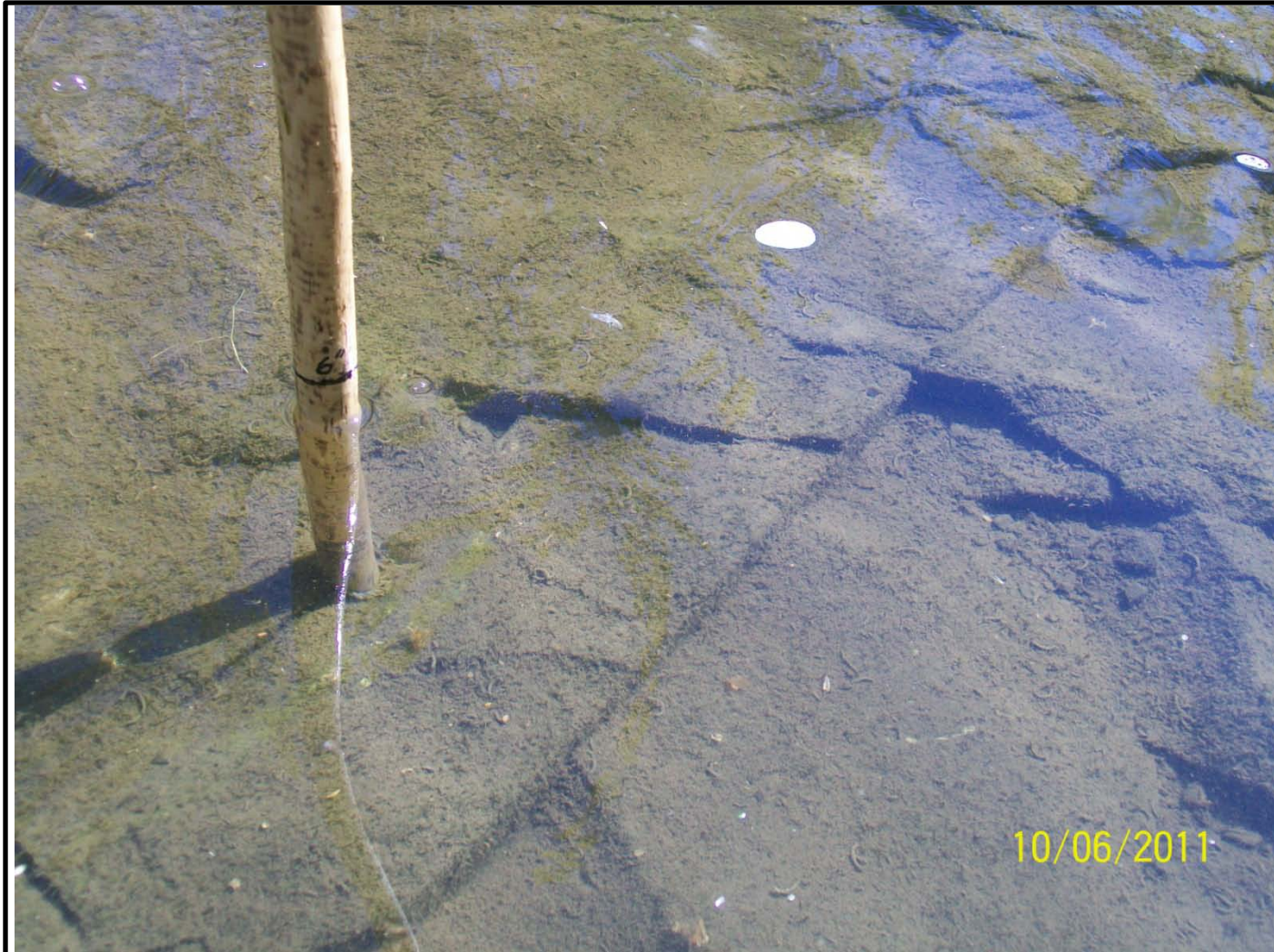
Photo #08 – Upstream of pooled area (Photo #06). Creek bottom is apparent bedrock with thin organic/sediment layer on rock surface. Water is approximately 5 inches deep; 6-inch mark on stick visible.
