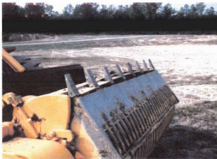
Figure 16. Blast Distortion (Bowing) to ROTAR ®
