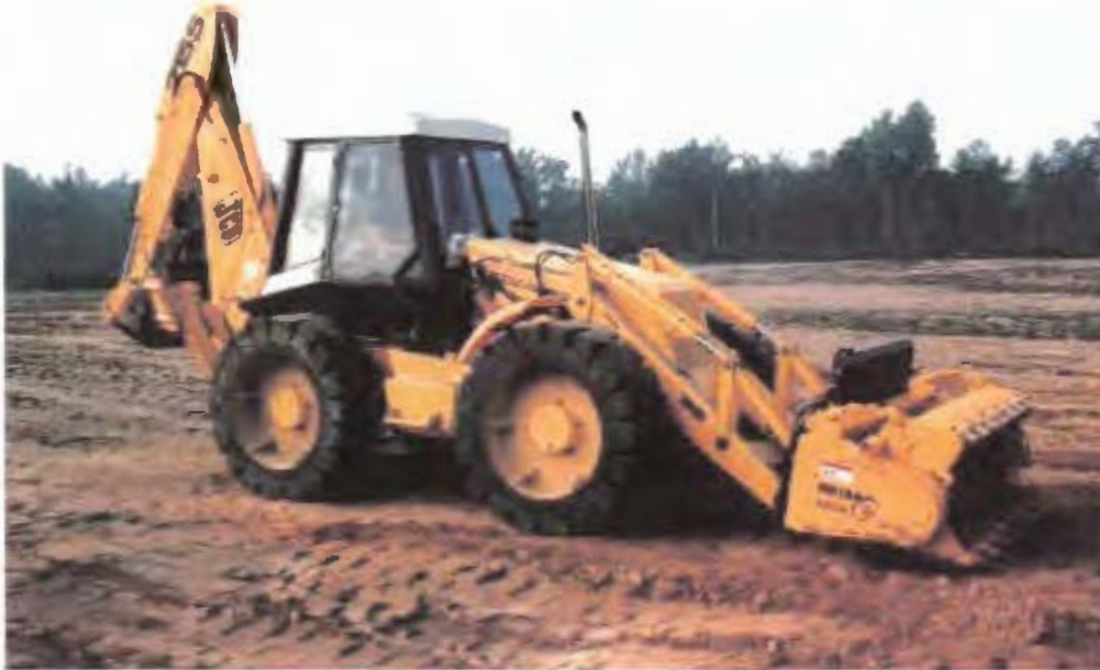
Figure 1. Improved Backhoe With HPL 800 S ROTAR ®
