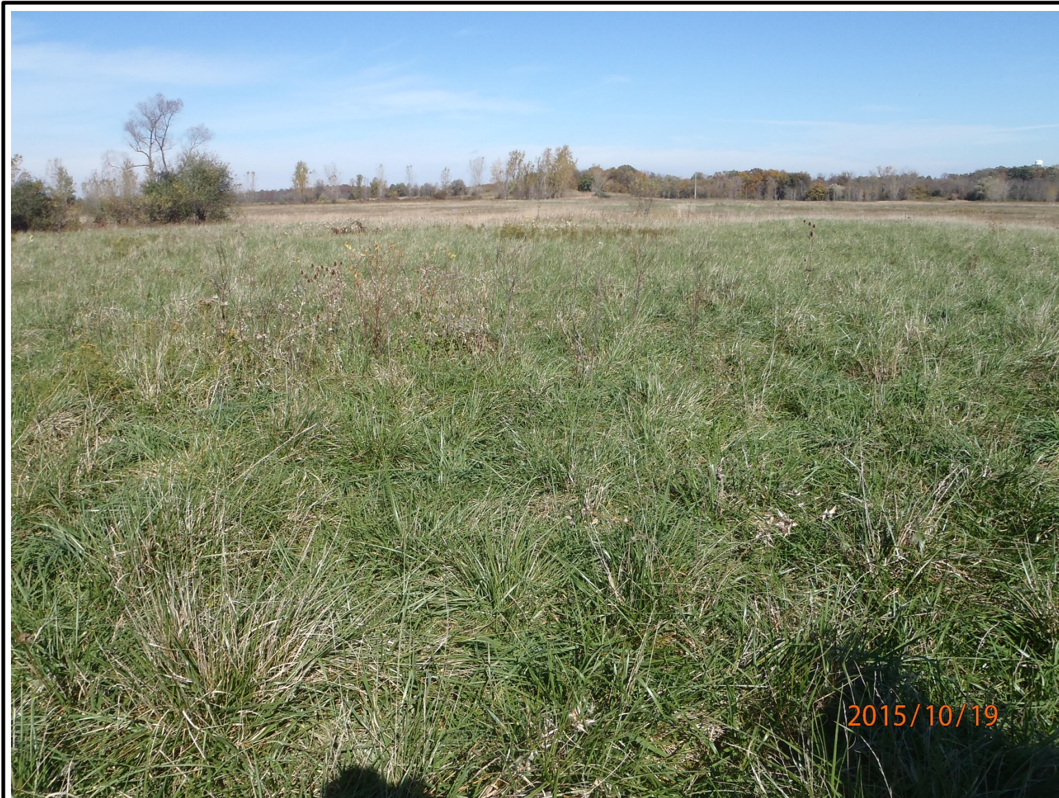
Photo #07 – Grid C2. No erosion or disturbances to the cap were observed. The grid is well vegetated. View to the northeast.
