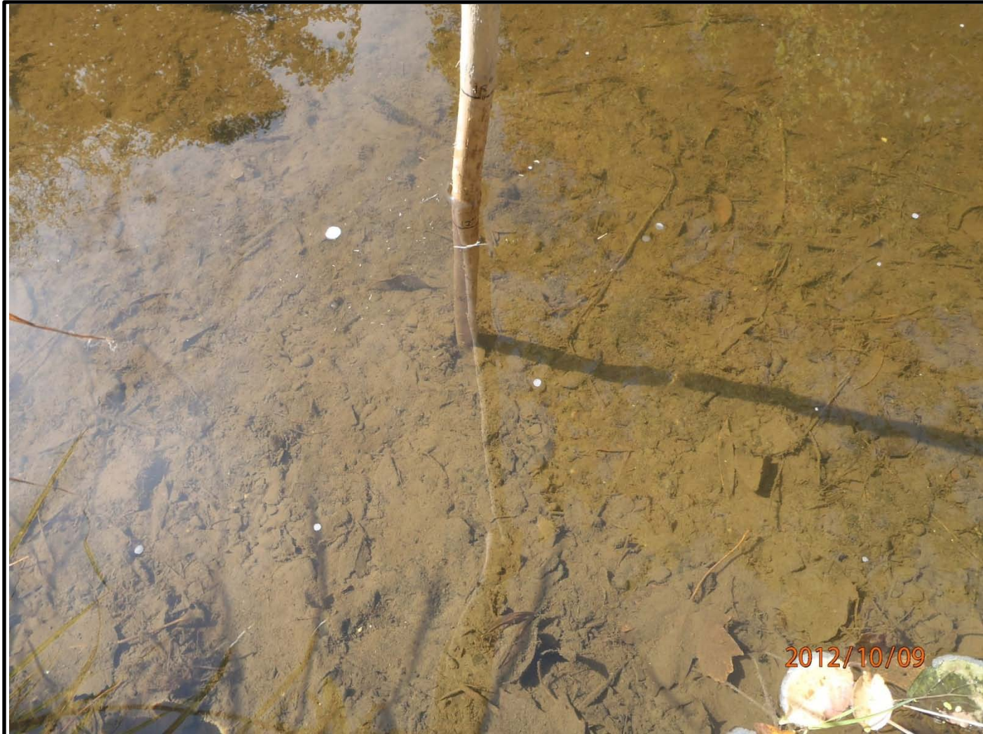
Photo #04 - Looking at Reeder Creek stream bottom. Creek bottom has small layer of sediment above fractured shale over apparent bedrock (shale). Sediment appears to be from decomposition than migration. Water is approximately 14 inches deep; 18-inch mark on stick visible. Sediment is about 2 inches deep
