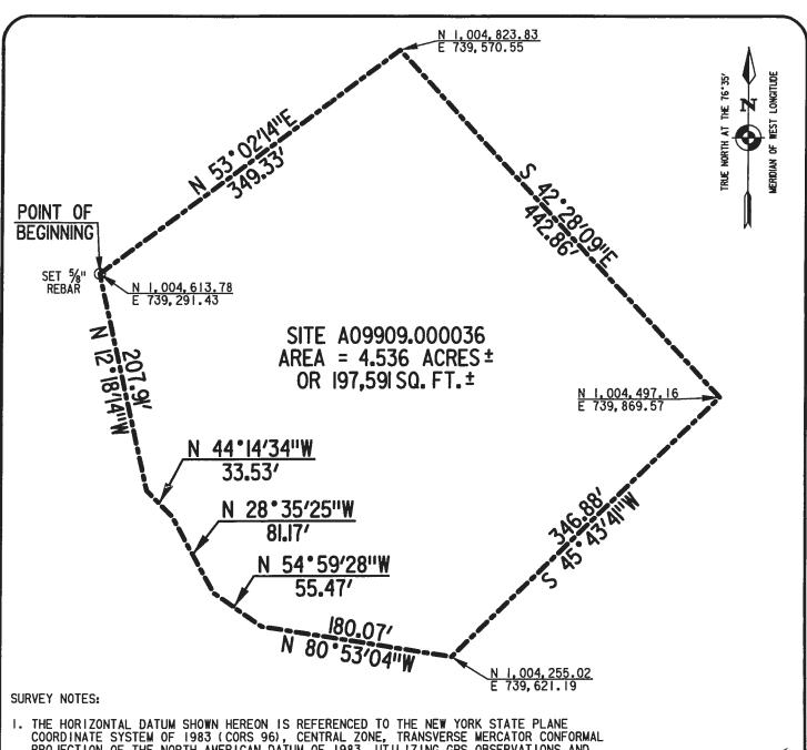
1. THE HORIZONTAL DATUM SHOWN HEREON IS REFERENCED TO THE NEW YORK STATE PLANE COORDINATE SYSTEM OF 1983 (CORS 96), CENTRAL ZONE, TRANSVERSE MERCATOR CONFORMAL PROJECTION OF THE NORTH AMERICAN DATUM OF 1983, UTILIZING GPS OBSERVATIONS AND THE NATIONAL MEMBERS OF SURVEY'S ONLINE USER POSITIONING SERVICE (OPUS) AND THE FOLLOWING MONUMENTS:
