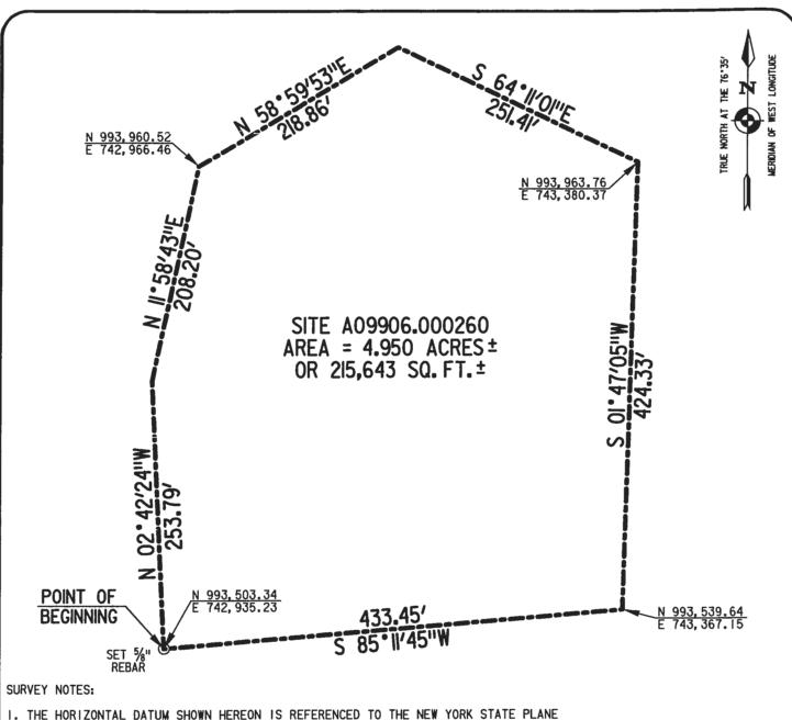
I. THE HORIZONTAL DATUM SHOWN HEREON IS REFERENCED TO THE NEW YORK STATE PLANE COORDINATE SYSTEM OF 1983 (CORS 96), CENTRAL ZONE, TRANSVERSE MERCATOR CONFORMAL PROJECTION OF THE NORTH AMERICAN DATUM OF 1983, UTILIZING GPS OBSERVATIONS AND THE NATIONAL GEODETIC SURVEY'S ONLINE USER POSITIONING SERVICE (OPUS) AND THE FOLLOWING MONUMENTS:
