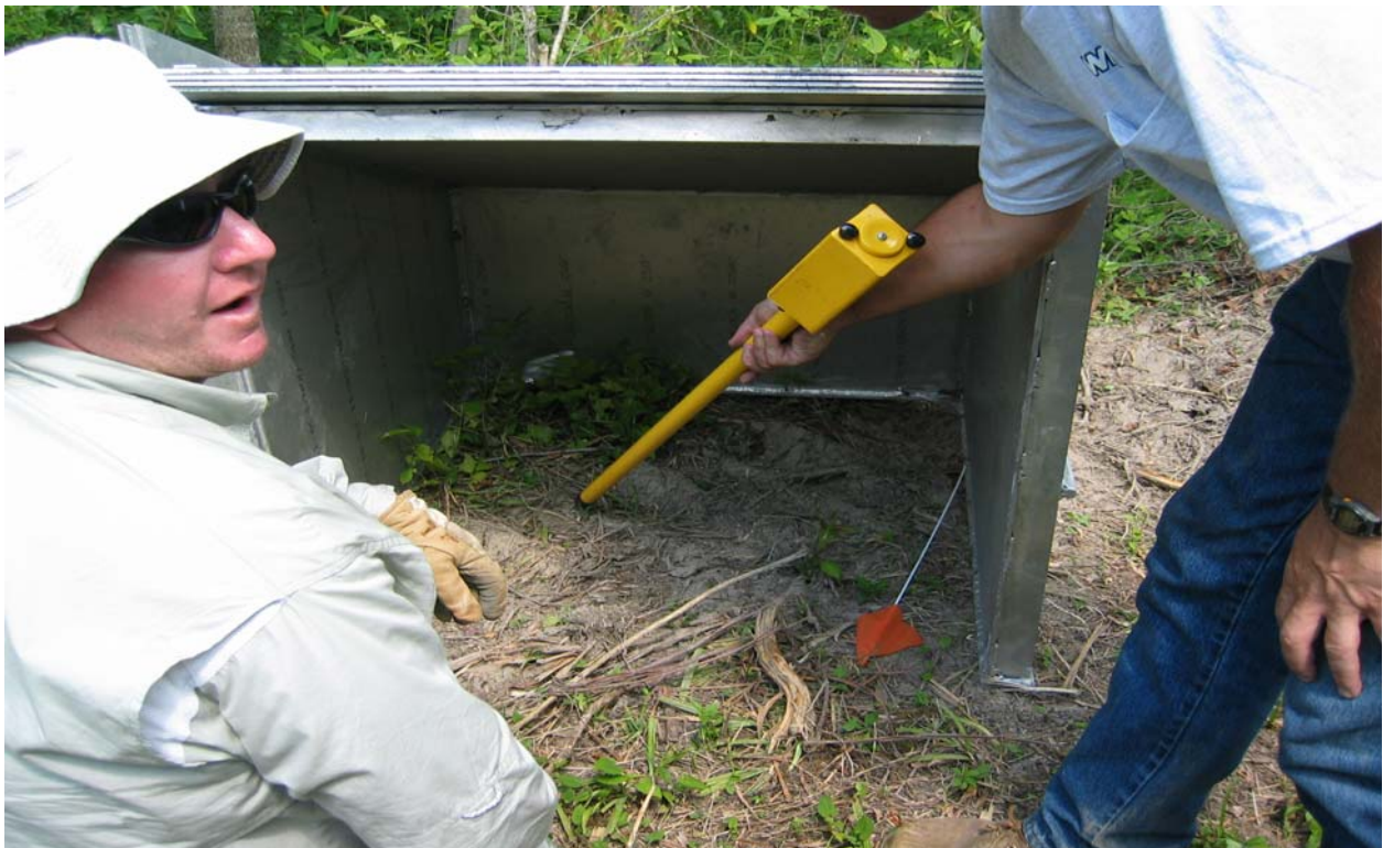
Photo No. 7: Anomaly reacquisition using a Schonstedt GA-52CXS ferrous metal locator and a miniature open front barricade (MOFB)
