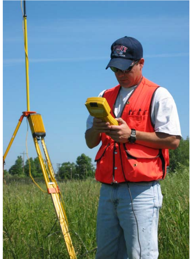
Photo No. 4: RTK Setup
