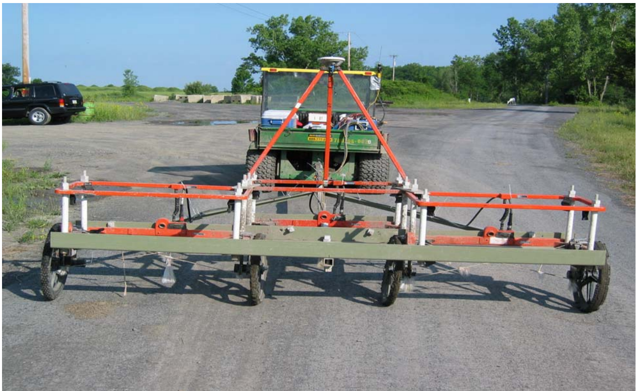
Photo No. 2: EM61-MK2 Towed-Array System (July 2003)
