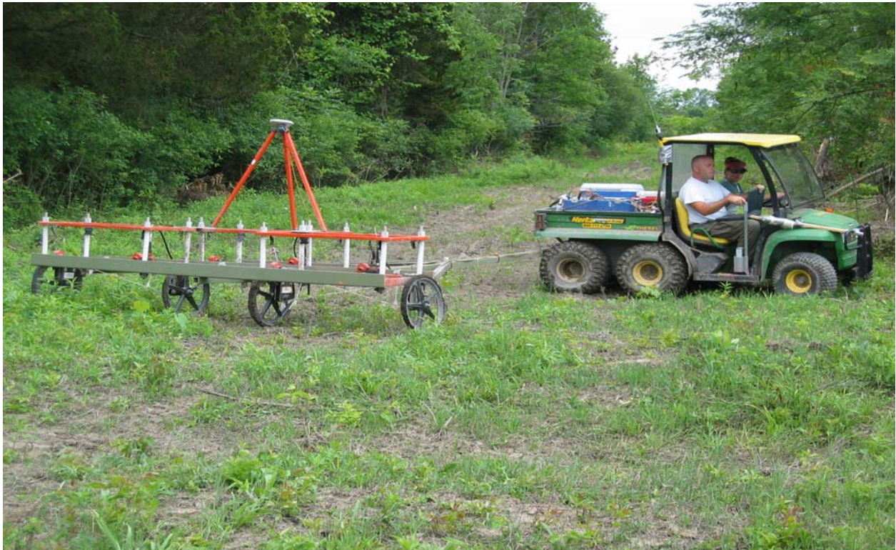
Photo No. 1: EM61-MK2 Towed-Array System (July 2003)
