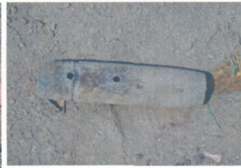
75mm Projectile after detonation of shaped charges
