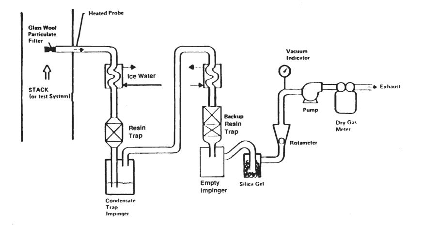
Figure 5-4: Typical Volatile Organic Sampling Train (VOST) Set-up
