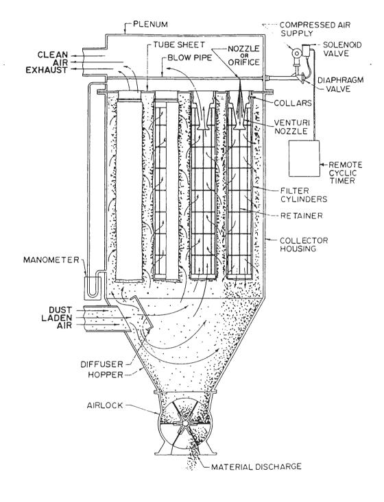
Figure 2-6 Baghouse Operation - Cutaway View
