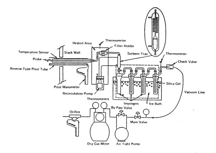
Figure 5-3: Typical Modified Method 5 (MM5) Train Set-up
