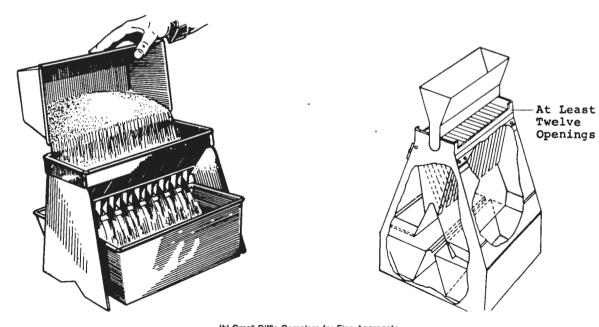
(b) Small Riffle Samplers for Fine Aggregate
