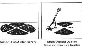
FIG. 2 Quartering on a Hard, Clean Level Surface
