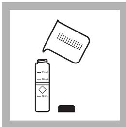
6. When the timer beeps, fill a sample cell with at least 10 mL of sample (the blank).
