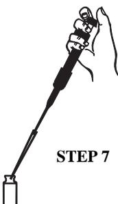
7. With the tip in contact with the side of the receiving vessel, slowly and smoothly press down on the turret cap until it reaches the stop and the solution is completely discharged.
