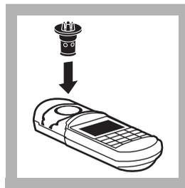
**15.** Insert the COD/TNT Adapter into the cell holder by rotating the adapter until it drops into place. Then push down to fully insert it.
