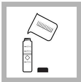
**6. Fill a second cell to the 10-mL mark with sample.**
