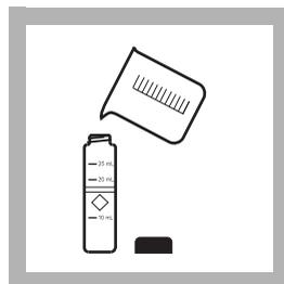
3. Fill a clean sample cell with 10 mL of sample (the blank).
