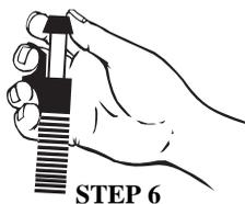
6. Use the thumb and forefinger to twist the turret cap to the next higher volume position to ensure quantitative transfer of the sample. The “F” position provides full blowout.
