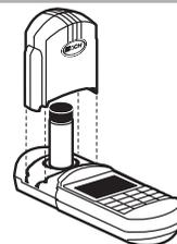
12. Within three minutes after the timer beeps, place the blank into the cell holder. Tightly cover the sample cell with the instrument cap.
