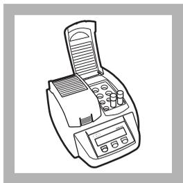
**10.** Cap the vial assemblies tightly and place them in the reactor for 2 hours at 103–105 °C.
