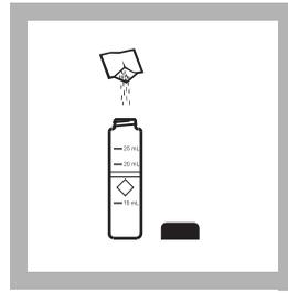
7. Add the contents of one DPD Free Chlorine Powder Pillow to the sample cell (the prepared sample). Cap the cell and swirl to mix.
