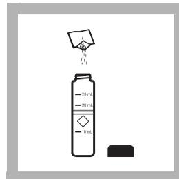
**4.** Add the contents of one NitraVer 5 Nitrate Reagent Powder Pillow to the sample cell (the prepared sample). Cap the sample cell.
