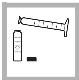
**5.** Transfer 25 mL of the prepared sample to a sample cell.
