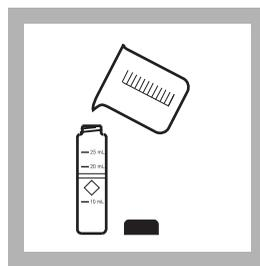
**3.** Fill a sample cell with 10 mL of sample (the blank).
