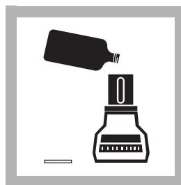
**3.** Homogenize 100 mL of sample for 30 seconds in a blender.
