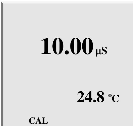
9. Use the **UP ARROW** or **DOWN ARROW** button to adjust the reading on the display until it matches the value of the calibration solution you are using.
