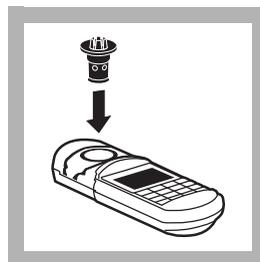
**3.** Insert the COD/TNT Adapter into the cell holder by rotating the adapter until it drops into place. Then push down to fully insert.
