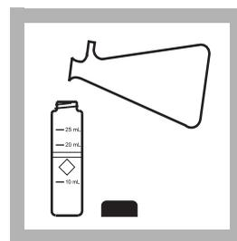
**8.** Fill a second sample cell (the prepared sample) with 25 mL of the filtered sample.
