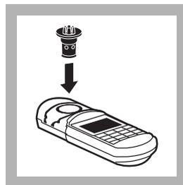
**3.** Insert the COD/TNT Adapter into the cell holder by rotating the adapter until it drops into place. Then push down to fully insert it.
