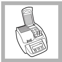
**6.** Place the vials in the Reactor. Heat for 30 minutes.
