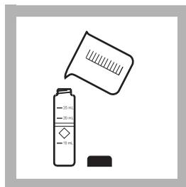
6. Fill another sample cell with 10 mL of sample (the blank). Clean the outside of the cells with a towel.
