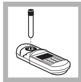
**16.** Place the **reagent blank** vial assembly in the adapter.
