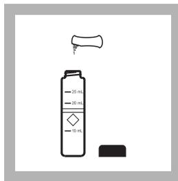
**7. Add the contents of one CuVer 1 Copper Reagent Powder Pillow to the sample cell (the prepared sample). Swirl the cell to mix.**
