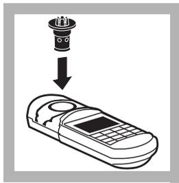
**9.** Insert the COD/TNT Adapter into the cell holder by rotating the adapter until it drops into place. Then push down to fully insert it.
