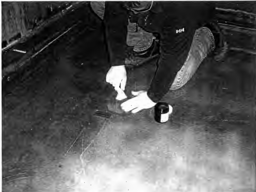
PCB Wipe sample Bldg 301.
