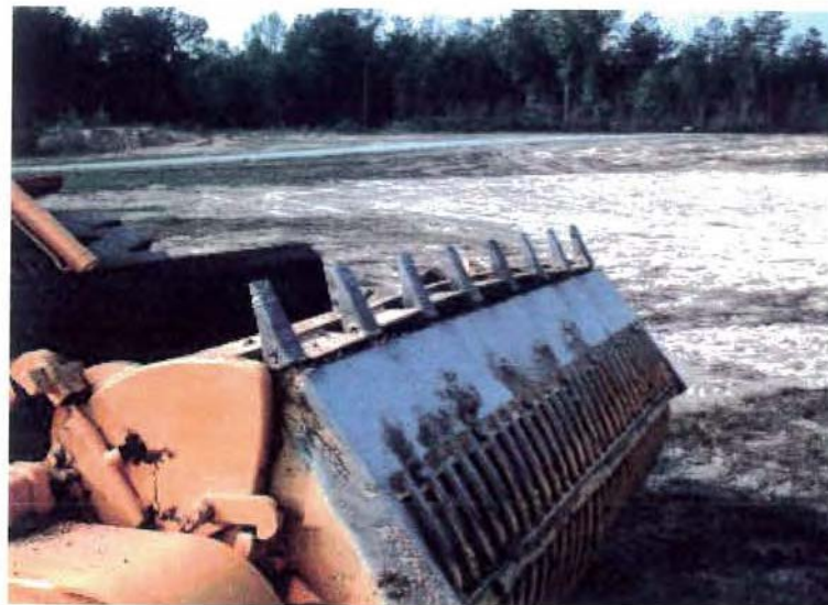
Figure 16. Blast Distortion (Bowing) to ROTAR ®
