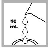
10. Fill a second sample cell with 10 mL of the reacted prepared sample.
