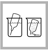
3. Prepare the sample: Collect at least 40 mL of sample in a 50-mL beaker. Fill the AccuVac Ampul with sample. Keep the tip immersed while the AccuVac Ampul fills completely.
