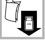
**9.** When the timer expires, insert the blank into the cell holder.
